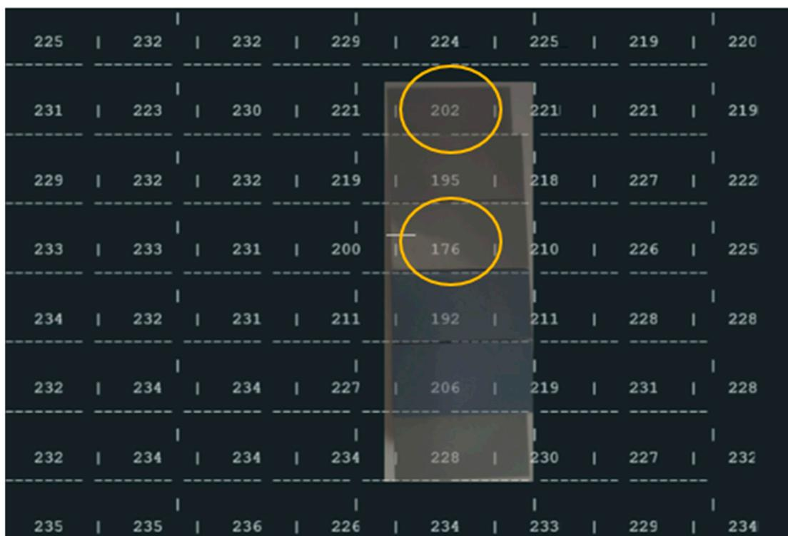
Figure 15. Results of the ToF sensor with the first block inside the office trash box (superposed images), yellow circle experimental values used to compare with real values.
