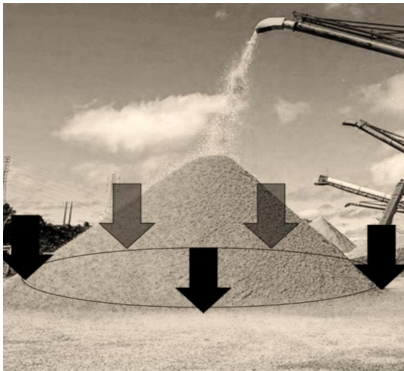
Figure 4. Diferent sampling points in the woodchips storage Where the moisture readings were registered with the calibrated dielectric meter.
