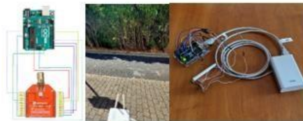
Figure 1. Electrical scheme of the transmission and LG02 gateway in the receiver.
