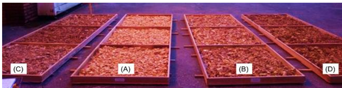
Figure 3. Experiment installation for woodchips drying: (C) Eucalyptus chips without bark; (A) Pinus chips without bark; (B) Pinus chips with bark and (D) Eucalyptus chips with bark.
