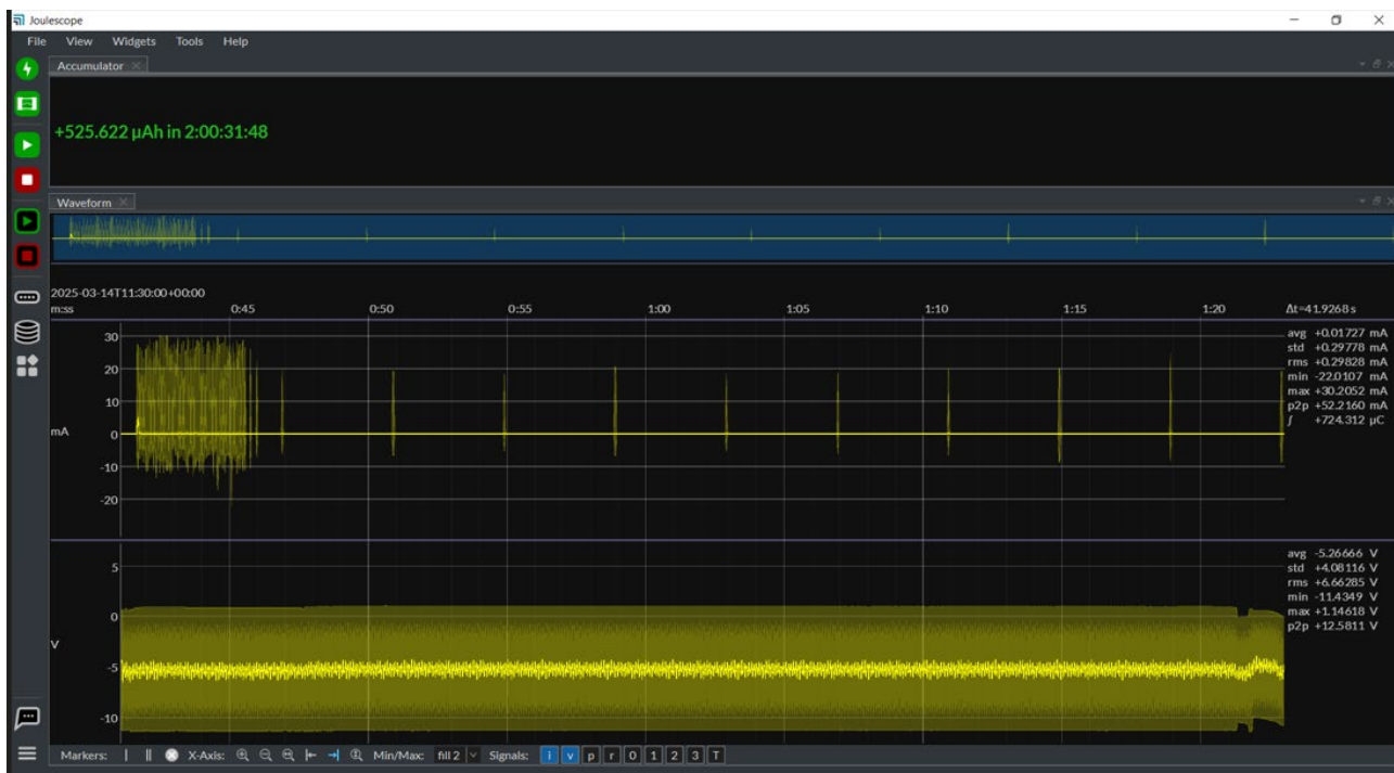
Figure 13. Energy consumption recorded for the IoT-Temp Node over 2 days.
