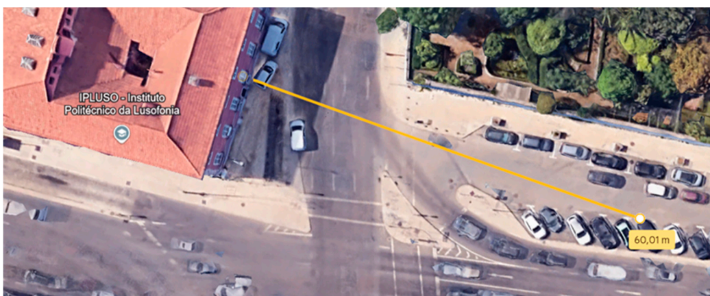
Figure 14. LOS scenario at 60m (GW at the window of the building and ED at the other side of the street in the parking lot).
