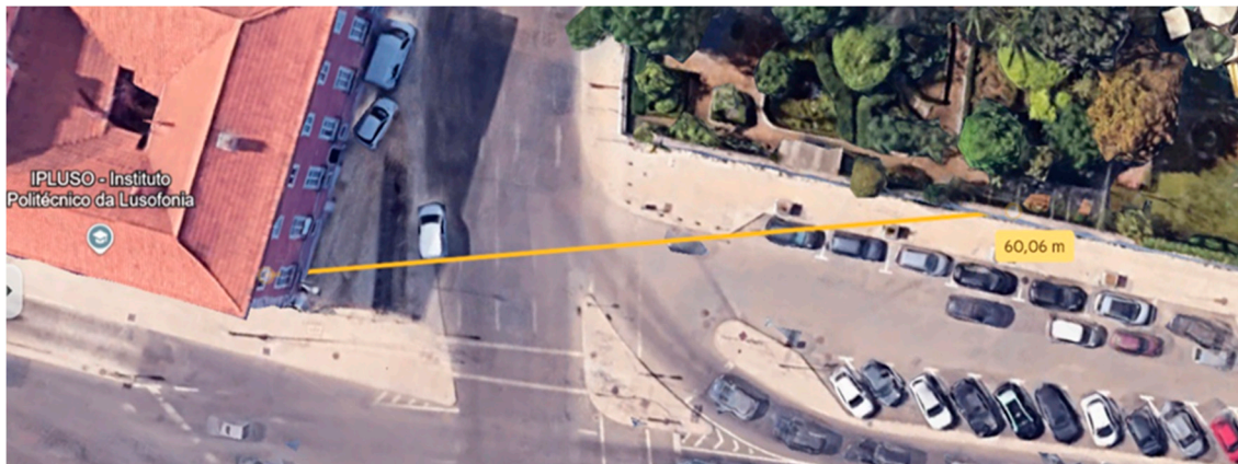
Figure 23. NLOS scenario at 60m (GW at the window of the building and ED at the other side of the street behind a concrete wall).
